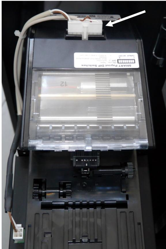
Lift the module out in a vertical upward direction.
