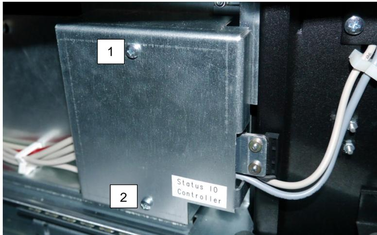
Remove the housing cover. Remove the connectors. Disengage the four tabs of the holders (see arrows) and carefully remove the controller.
