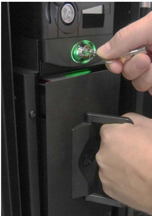
Press the locking device in the direction of the arrow to the right and remove the safebag from the holder.
