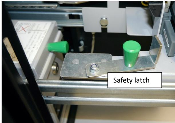
Pull out the support until the latch (1) easily hooks into the slot in the housing (2).
