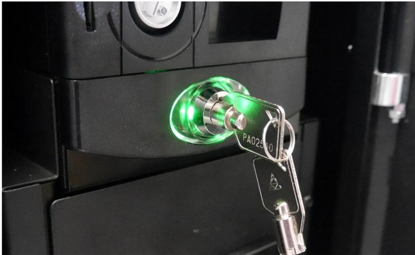
Hold the key in this position, grasp the module at the handle and pull it out to the front.
