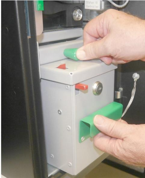
The cassette is locked after being removed and can only be opened with the coin box key.
