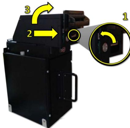
Then pull the module to the front (2) and take out of the case (3).
