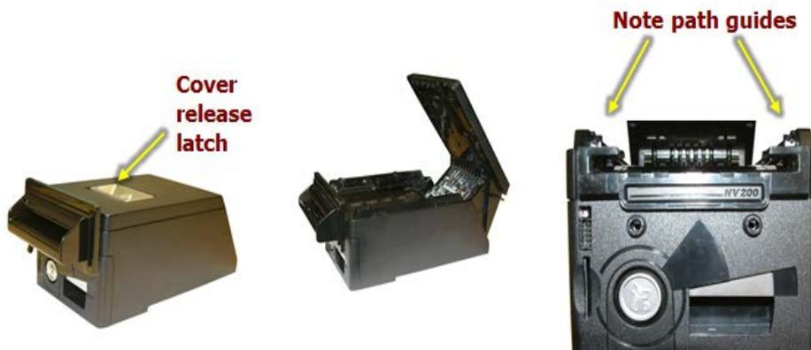
The note path is now visible and can be cleaned. Carefully clean the surface with a soft, lint-free cloth moistened with water and mild detergent. (Such as Diebold Nixdorf Multi-Media-Cleaner 01750035530) – Be extra careful while cleaning the lenses (sensors) and make sure they are clean and dry before closing the cover and restarting the unit.
