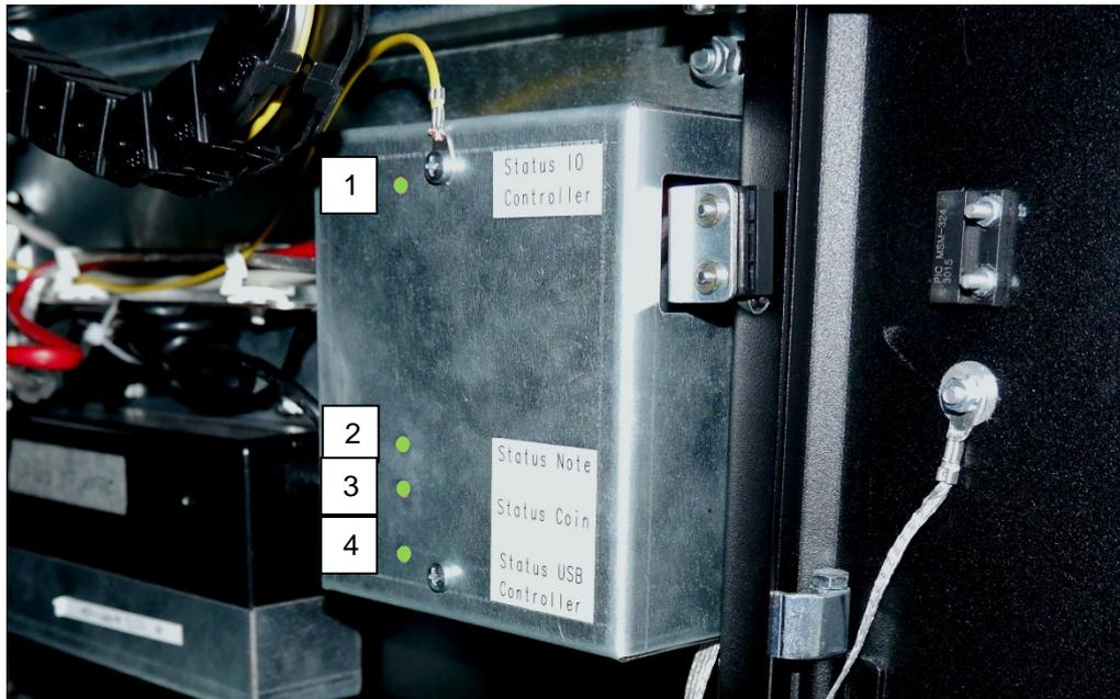
During system initialization, the I/O interface module runs through the different colors (red, yellow, green) on the LED panels for a visual LED check.
